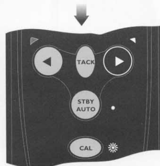
Fig 3.5 - Increasing Gain level
