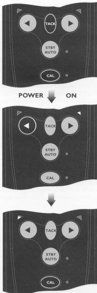
Fig 3.2 - Configuring for Port mounting
